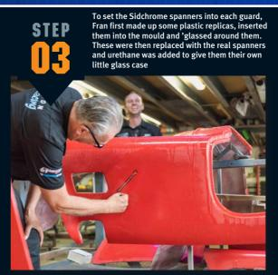
The body is made up of 17 separate pieces that will be bonded together prior to paint. Once the body is bonded to the chassis it would have to be cut off to remove it, which is why the boys are so fastidious during the build process
