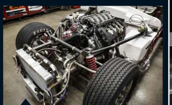
Finally we have our intake manifold, so Joe can begin fabricating the cold-air intake, or as he calls it, 'the elephant's trunk'. The radiator is one of Aussie Desert Cooler's finest, naturally! The worm-drive wiper motor sits on top of the passenger footbox, out of harm's way
